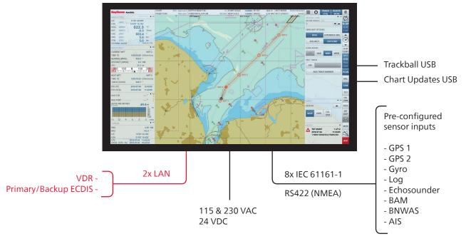
In case of a legacy Raytheon Anschütz ECDIS 24 installation, the magicplex can still be used and easily connected via LAN to the new panel-pc.
